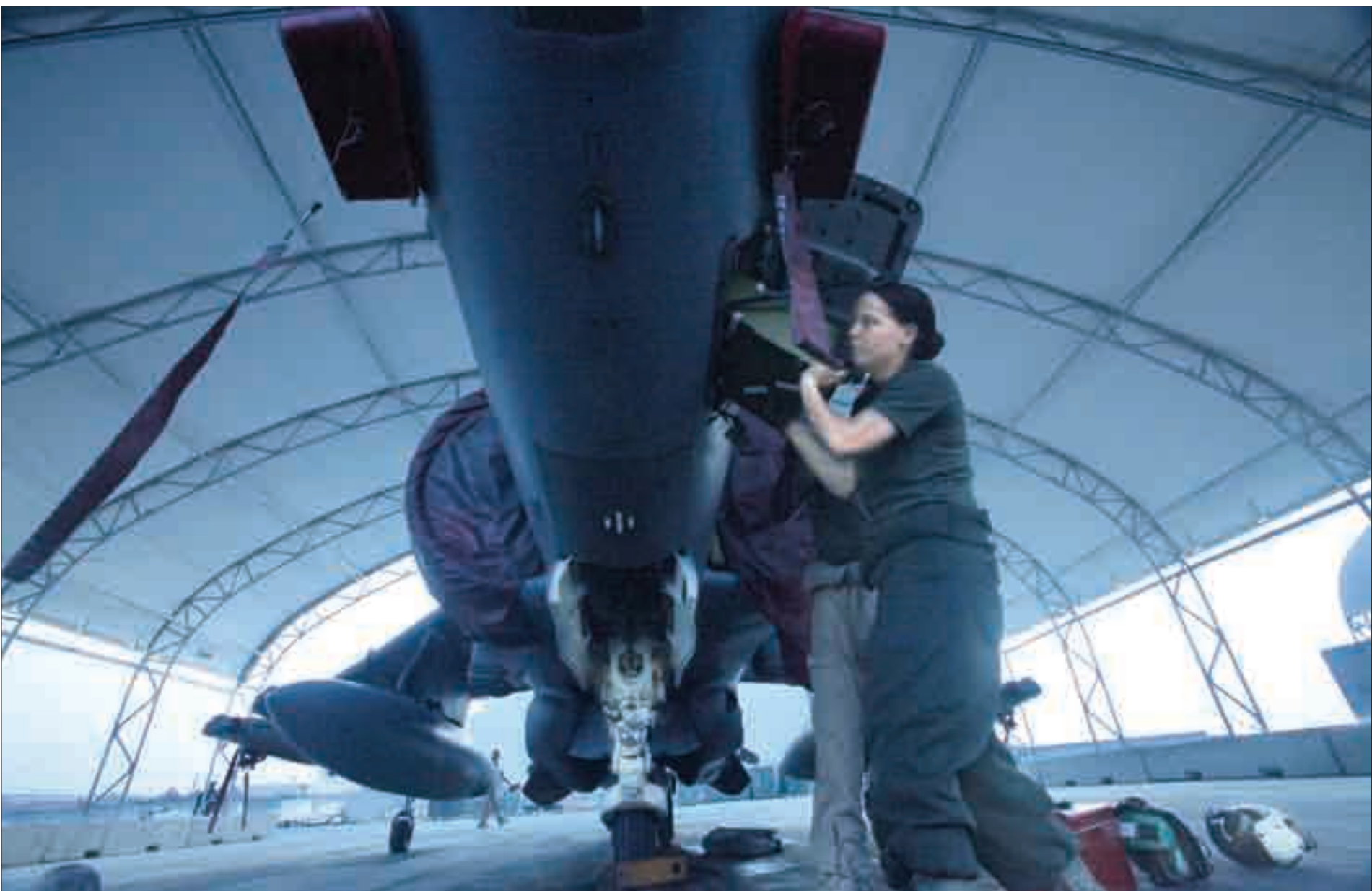
Cpl. Ashley Zifko, a Marine Attack Squadron 513 avionics technician and Two Rivers, Wis., native, installs an inertial navigation unit on one of the AV-8B Harriers on the flight line at Kandahar Airfield, Afghanistan, Aug. 9.
