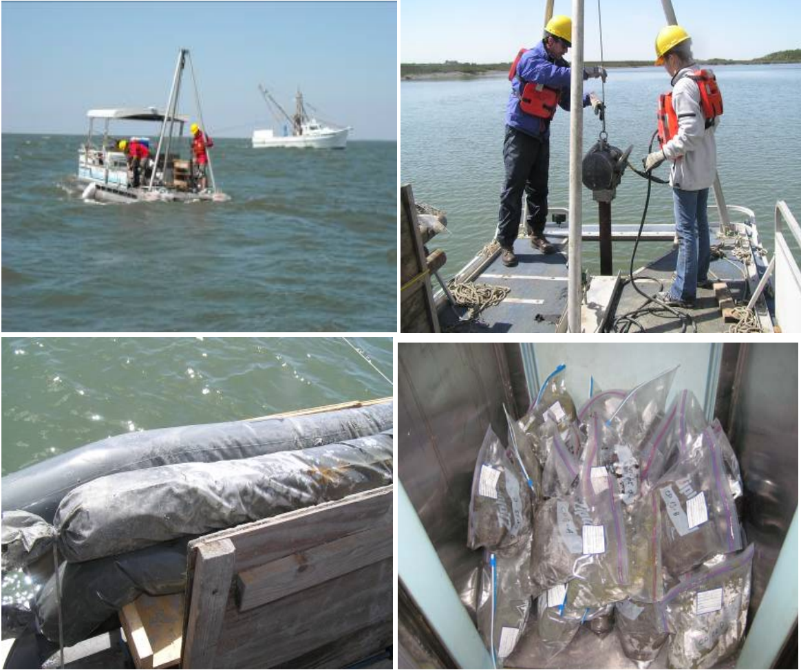
Figure 3. Pontoon boat retrofitted with vibracore (upper left); deploying the vibracore (upper right); vibracore samples in plastic liners (lower left); 1-foot vertical sections of sediment ready for shipment to analytical laboratory (lower right).
